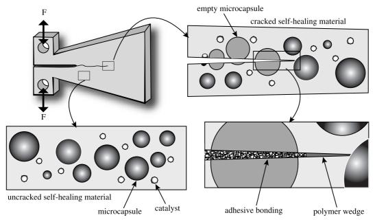
Figure 1. Details of the self-healing process during fatigue.
